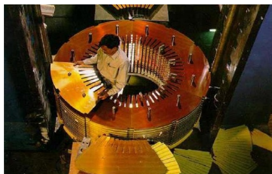
Fig. 4: Manual assembly process [4]
